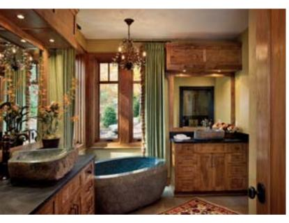
Because of the enormity of the boulder bathtub – 3,500 pounds – special care had to be taken. "We built a pedestal where the tub would be, flew the tub in on a crane and put a box around it," says homeowner and builder Brett Schwebke. "Then we basically built the whole house around the tub."
